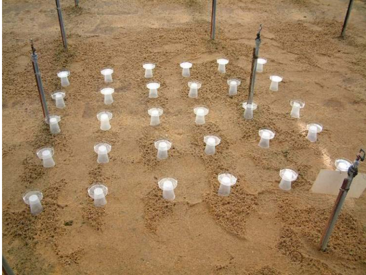
Photo 5. Testing mist distribution uniformity at New Place Nurseries, September 2007
