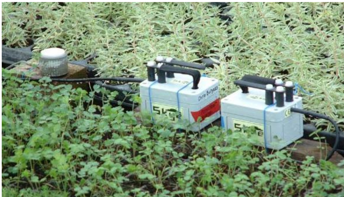
Photo 4. One Evaposensor linked to Nobel or ETS interface to control mist burst frequency and the other Evaposensor connected to logger to monitor environment achieved. PAR quantum sensor to record light levels also shown.
