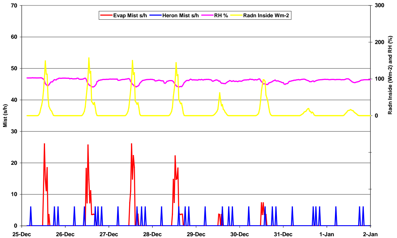
Fig 7. Lowwaters. Half-hourly means. Misting restricted to bright periods only in winter from Evaposensor control compared to regular timed bursts of mist during the day from under Heron timer control.
