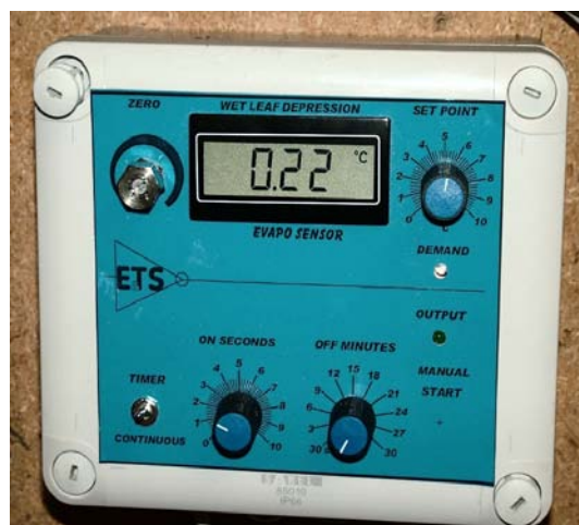
Photo GS2. Evaposensor (Skye) and Evapomist controller (ETS)
