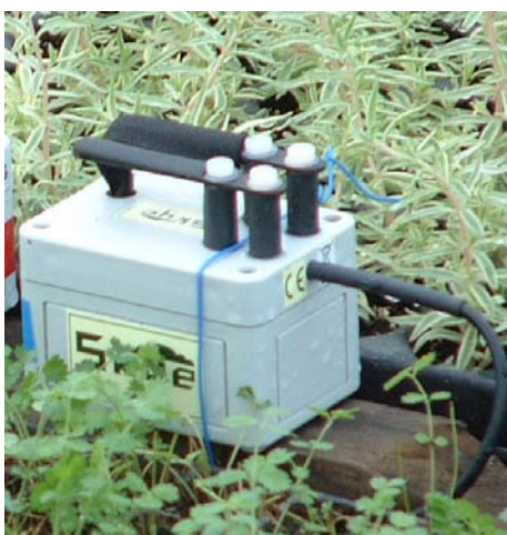
Photo GS2. Evaposensor (Skye) and Evapomist controller (ETS)
